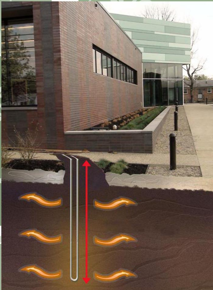
Geothermal heating and cooling uses stored underground heat – naturally renewable and non-polluting – to heat and cool the building. A geothermal heat pump can move more than three units of heat energy for every one unit of electrical energy used to power the system. A SMART control allows air flow to create a more comfortable atmosphere for people.
