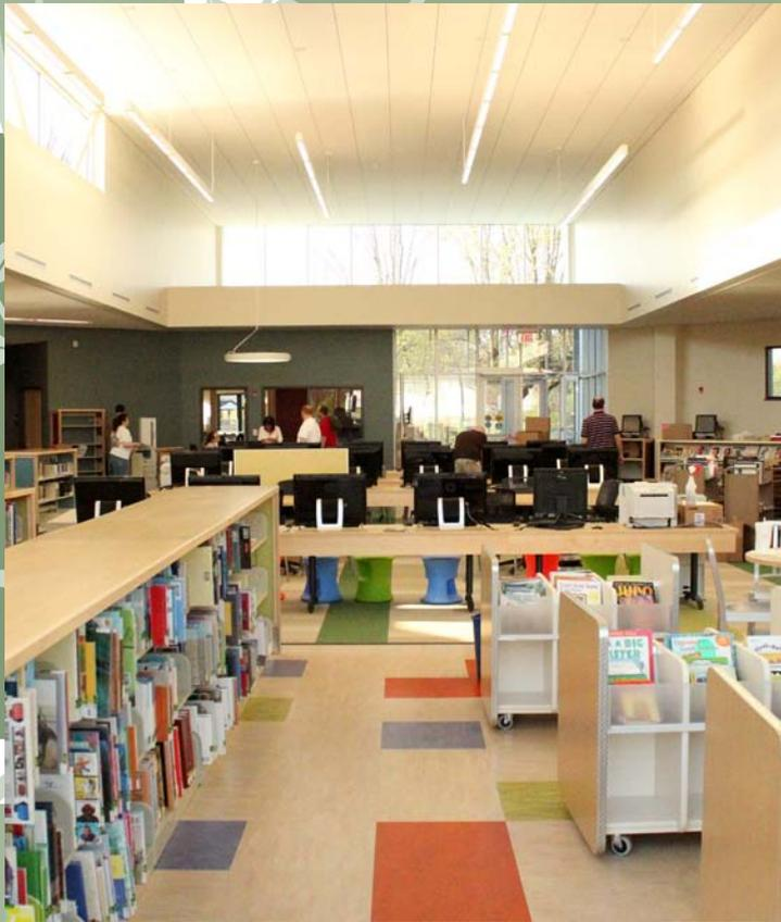
Electronic eye sensors detect the amount of light coming through windows into the building and adjust indoor lighting, making it brighter or dimmer as needed. This saves energy and allows for a more comfortable atmosphere inside the library. Lighting is also directed toward specific areas allowing it to be used effectively.
